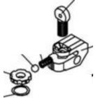
We recommend using the TS211 sight adjusting tool, but you can use a pointed object like a bullet tip or a hardwood dowel. Rotate the elevation dial CW so that the aperture is being raised. Continue to rotate the dial until the aperture is all the way up and falls out of the sight. Then the elevation dial and washer will come out and the small detent ball will be free to fall out.
