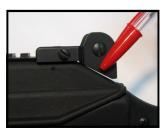
10. While using a flat headed screw driver to tighten the cross screw, swing the rear of the sight left and right (perpendicular to the rail). Swinging the rear of the sight while tightening the cross screw will help "seat" the sight on the synthetic rail.
