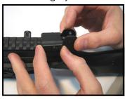
9. Looking from the side, grasp the sight and slide it forward until it lightly touches the rear sloping area of the receiver.
