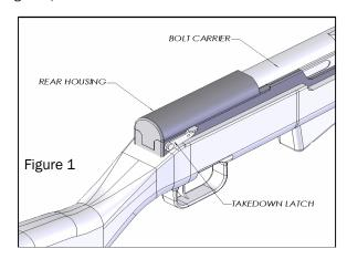
3. Remove the Takedown Latch. This will require the Latch Pin to be removed from the Takedown Latch. On some SKS models the Latch Pin is pressed into the Takedown Latch. On other rifles the Latch Pin is brazed in place. (Consult a gunsmith if you find that you cannot remove the small Latch Pin from the Takedown Latch.) Note: Some models may fall under BATF Curio & Relic restrictions, please check to see if your rifle can be modified under these guidelines. (See Figure 2)
