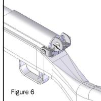
Adjusting Hint: A piece of notebook paper inserted between each adjusting screw and the receiver will work as a feeler gauge to let you know when the screw is getting close to the receiver. When the set screw begins to clamp on the paper, remove the paper strip and tighten 1/8 of a turn. This will get things tight without over tightening. (Repeat for the 3 additional adjusting screws).
