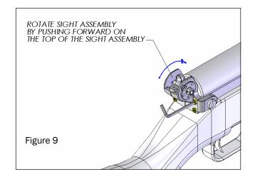
12. Using a coin edge (penny) tighten the Cross Screw until the Sight is drawn tight against the right side of the Receiver. Check the stability of the Sight by pushing forward and back on the top of the Sight Assembly. Continue to slowly adjust the Screws until the Sight Assembly no longer moves.
