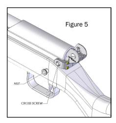
9. Thread the cross screw into the nut and continue to tighten the cross screw until the Sight Assembly is drawn tight to the right side of the Receiver. At this point the Sight Assembly should be snug against the right side of the Receiver, but still able to rotate on the Cross Screw. (See Figure 6)
