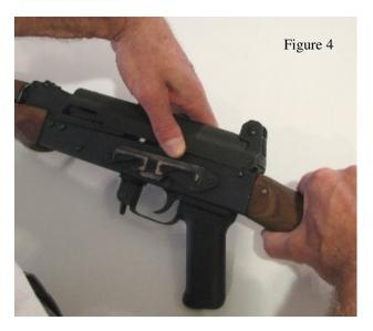
4. With the two detents disengaged the cover can now be slid back and out of the cover retention groove on the front of the receiver. Keeping the detent holes in the cover just below the detents, pull the cover ahead and off the rifle.
