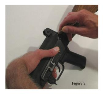
2. While squeezing firmly down on the cover, depress the detent with a pointed object until the cover disengages and drops slightly down below the detent.
