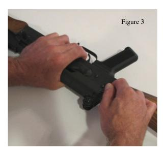
3. Continue firm steady pressure on the cover to hold it in position while you roll the rifle with the ejection port side up and depress the cover detent on that side until the cover disengages the detent and drops slightly below the detent.
